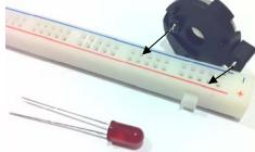
**Connect an LED** by pushing the anode (longer leg) into a tie on the red (+) strip and the other leg (the cathode) into the blue (-) strip. The two legs of the LED create a second connection across the two strips.
