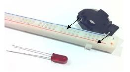
**Connect an LED** by pushing the anode (longer leg) into a tie on the red (+) strip and the other leg (the cathode) into the blue (-) strip. If all your connections are tight, you should see the LED light.
